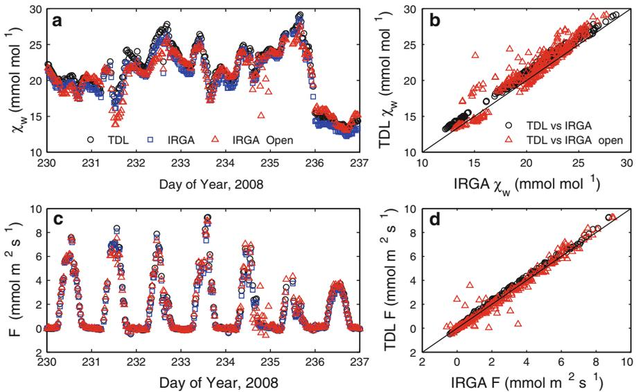
Fig. 8 Time series of water vapour mixing ratio measured with the TDL, IRGA, and open-path IRGA (and their 1:1 comparison); time series of the water vapour flux measured over the soybean canopy using eddy covariance based on three methods including the TDL, IRGA, and open-path IRGA (their 1:1 comparison)
