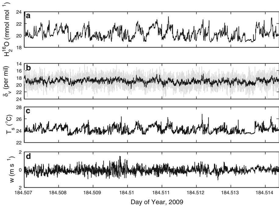
Fig. 5 Time series of high frequency (10 Hz) fluctuations of a  $H_2^{16}O$  mixing ratio; b oxygen isotope composition of water vapour; c sonic temperature; d vertical wind velocity. The gray trace in b represents the calibrated 10 Hz signal. The black trace shows the effect of adding a low pass (1-s running mean) filter
